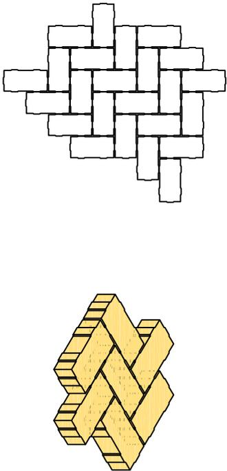
1 Plan and Isometric View of Porous Surface - Permeable Concrete Blocks
