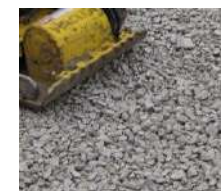
CGA type 4/20 (Clean stone) - permeable
