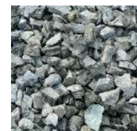
CGA type 4/20 (Clean stone) - permeable
